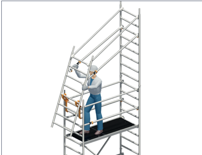
1. Attach the first ladder frame. Attach the Uni assembly hooks and position the second ladder frame in order to fit the guardrails and the Telescoping Guardrails as intermediate rails.
